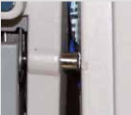
Figure 1: Backed out pivot latch screw
